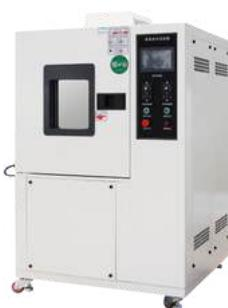
The Ozone Tester – Ozone Chamber simulates and intensifies ozone conditions to assess rubber's resistance to ozone-induced aging. It quickly identifies rubber's susceptibility to cracking and the effectiveness of anti-ozone agents, improving product durability.
