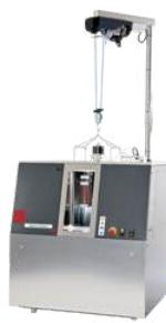
The Ozone Test Chamber – OzoneTest UV measures rubber's resistance to cracking under static or dynamic tensile strain, conforms to ASTM, ISO, DIN, and other international standards. It measures the resistance of rubber samples to cracking when subjected to static or dynamic tensile strain.
