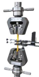
The Clip-On Extensometer is designed for testing rigid plastic, metal, and materials with elongation below 50%.
