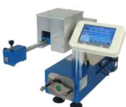
The QualiRebound-GB evaluates the resilience of elastomers within a hardness range of 30 to 85 IRHD points conforming to ASTM D7121 and ISO 4662 standards.
