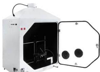
The UL 94 Flammability Chamber, also known as the Horizontal Vertical Flame Chamber, is specifically designed for testing the flammability of plastic materials used in electrical devices and appliances. It complies with several international standards, including ASTM, ISO, and IEC standards.
