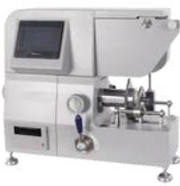
The QualiRebound-RDA Rebound Resilience Elasticity Tester measures elastomers' rebound resilience using a pendulum method and pneumatic clamping for accuracy.
