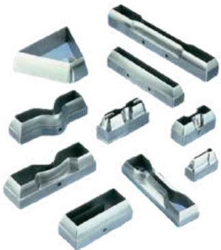
Specimen Dies and Molds are essential tools for preparing accurate test specimens that meet international testing standards such as ASTM, ISO, DIN, and JIS. Manufactured from hardened P20 tool steel, these dies are ground, polished, and optionally chrome-plated with Teflon coating to ensure durability and precision. The cutting edges are wire-cut from solid tool steel and designed for re-sharpening, allowing long-term, cost-effective use while maintaining high accuracy.
