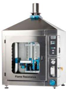
The Flammability Tester for Rubber and Plastics is designed to assess the flame resistance of rubber and plastic materials as per UL 94 standards. It conforms to ASTM, ISO, and other international standards. It features a stainless steel cabinet with a tempered glass viewing window, a Bunsen burner, and a precise gas flow meter.
