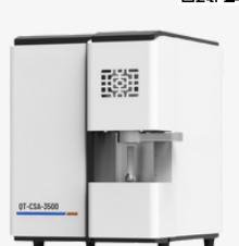
The QT-CSA-3500 ensures efficient combustion for accurate results, while the QT-CSA-3500G adds dual furnace flexibility with high-frequency induction and resistance furnaces, expanding application versatility.
